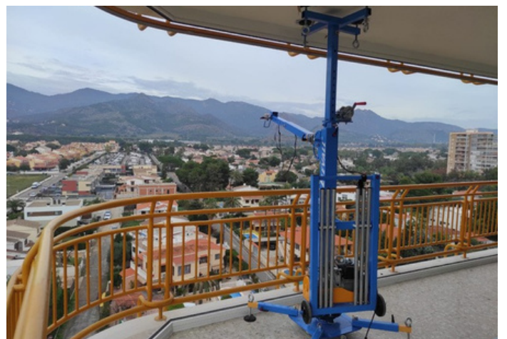
Balcony lifting with self-contained anchorage system
