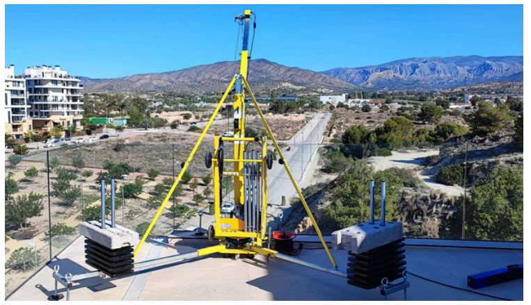
Two lifting capabilities, using self-contained anchor system or counterweights
